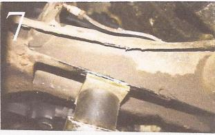
Mark the chassis where the weld-in brackets meet the frame horns.
