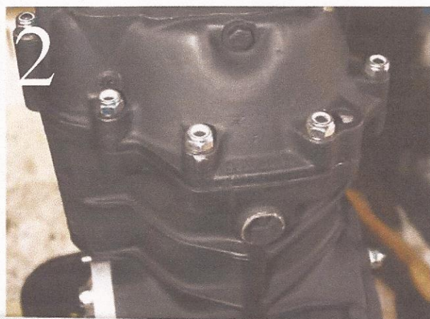
2 Standard gearboxes are bolted together with nuts on studs. Aftermarket gearboxes are often assembled with nylocs.
