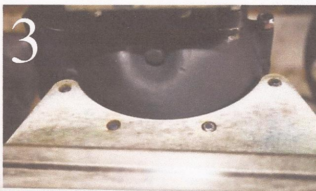
3 Either way, the studs aren't long enough to mount the mid-mount as shown here;
