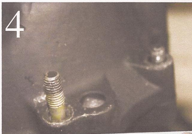
4 Remove the lower four nylocs and extract the studs. The mid-mount comes complete with longer bolts.
